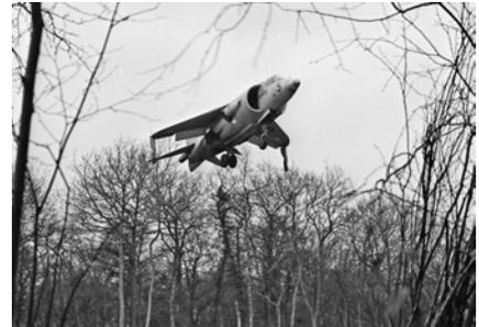
During 1975/76, the VIFF project (Vectoring in Forward Flight) assessed the benefits of using thrust vectoring in air combat. Harrier GR1 XV277 flew in one-on-one air combat over the RAE tracking range at Aberporth, off the Welsh coast. One hundred recorded one-on-one combats, each lasting three minutes, against an RAE Hawker Hunter and an RAF English Electric Lightning, were flown. The fruits of this work were seen a few years later, in the Falklands conflict.
