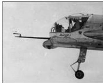
*Short SC1 XG905 in the hover Nov 1962, with small nose pod fairing and "Short SC1" label well forward.*
